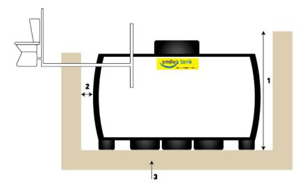
Excavate so that the depth provides cover over the top of the tank that is a minimum of 6" and a maximum of 30". Allow space of 18" to 24" on both sides of the tanks.
